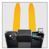
Controls and additional display in load direction (optional)
